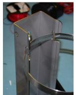
Slide the tamtorque through the two gaps in the bracket and then around the post to which the sign is being fixed onto
