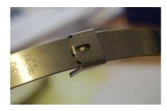
Begin by making sure that a small clip is found on the tamtorque fixing
